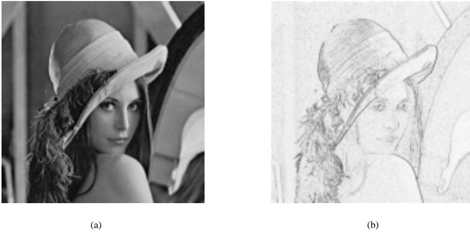
Fig. 7. Edge detector filters applied on Lena: (a) Original greyscale picture, (b) Edge detector local energy determined by edge detection (darkness represents high values).
