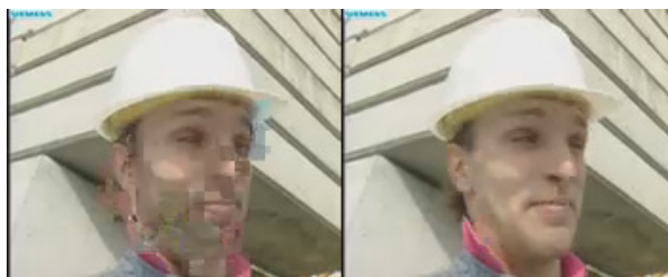
Figure 2.9 Picture number 15 from the sequence FOREMAN. Quality obtained with WIFI traces, with hard decoding on the left and soft decoding (forbidden interval of 0.09, W = 32 ) on the right.
